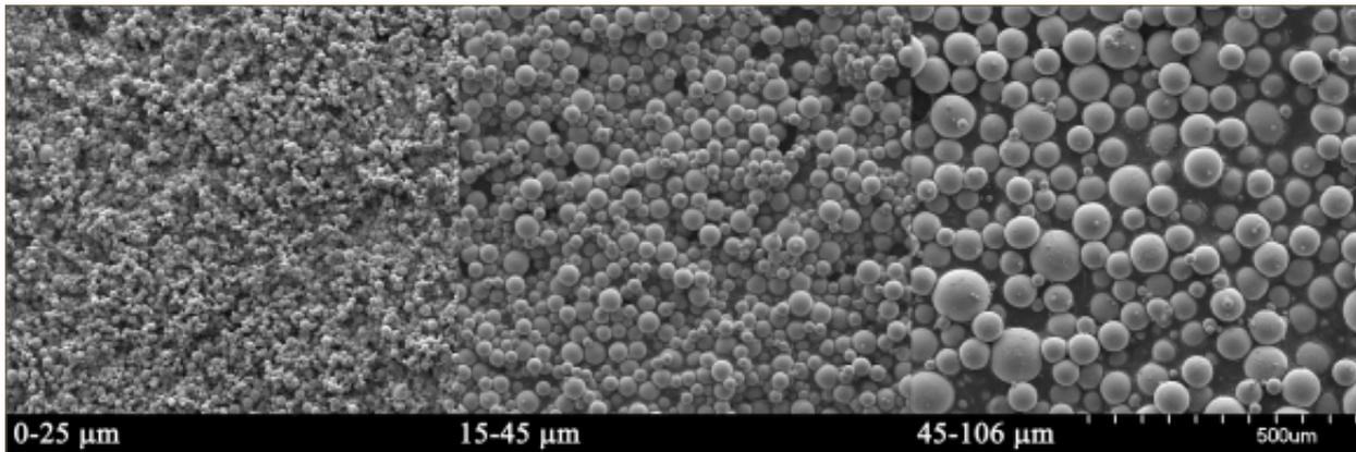
Fig. 6 SEM's of AP&C's (left) 0-25 µm powder, (centre) 15-45 µm powder and (right) 45-106 µm powder
