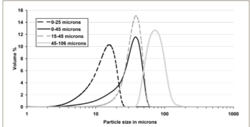
Fig. 5 Laser diffraction measurements of the particle size distribution of Ti-6Al-4V ELI powders produced via plasma atomisation
