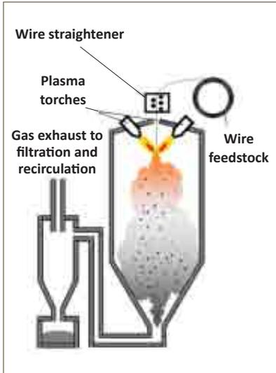
Fig. 2 Schematic of the plasma atomisation setup
