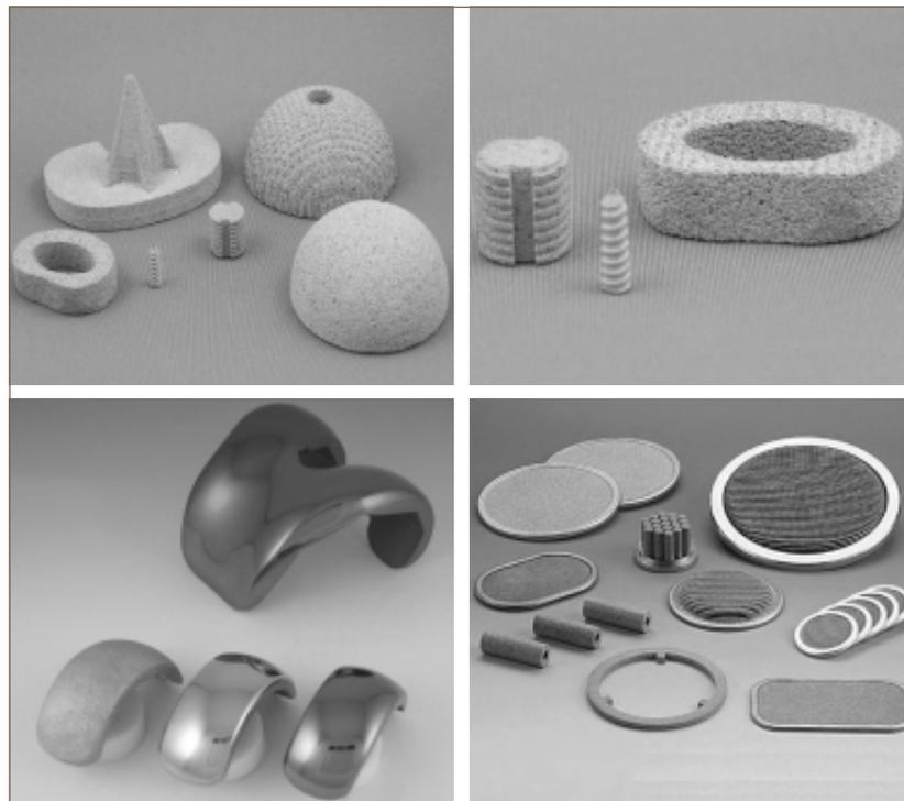
*Fig. 1 Products made from AP&C's titanium or titanium alloy powders. Top left and top right: Titanium orthopedic parts for hip joint replacement made via MIM; Lower left: titanium knee implant parts made via PIM; Lower right: titanium filtering media*
